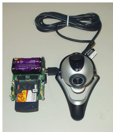
Fig. 3. Stargate board interfaced with a medium resolution camera. Stargate hosts an 802.11 card and a MICAz mote that functions as a gateway to the sensor network.
