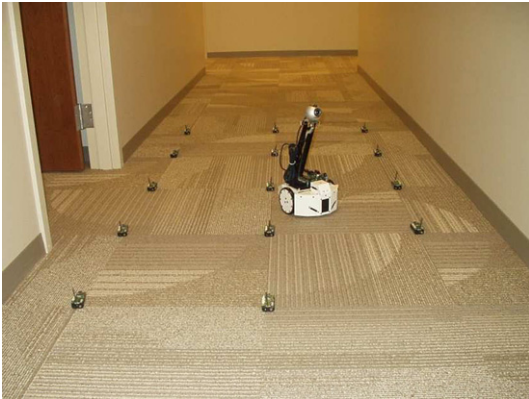
Fig. 5. GARCIA deployed on the sensor testbed. It acts as a mobile sink, and can move to the area of interest for closer visual inspection. It can also coordinate with other actors and has built-in collision avoidance capability.
