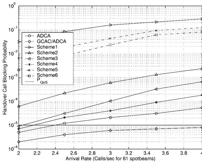
Figure 12. The handover call blocking probabilities ( $C = 190$ ).
