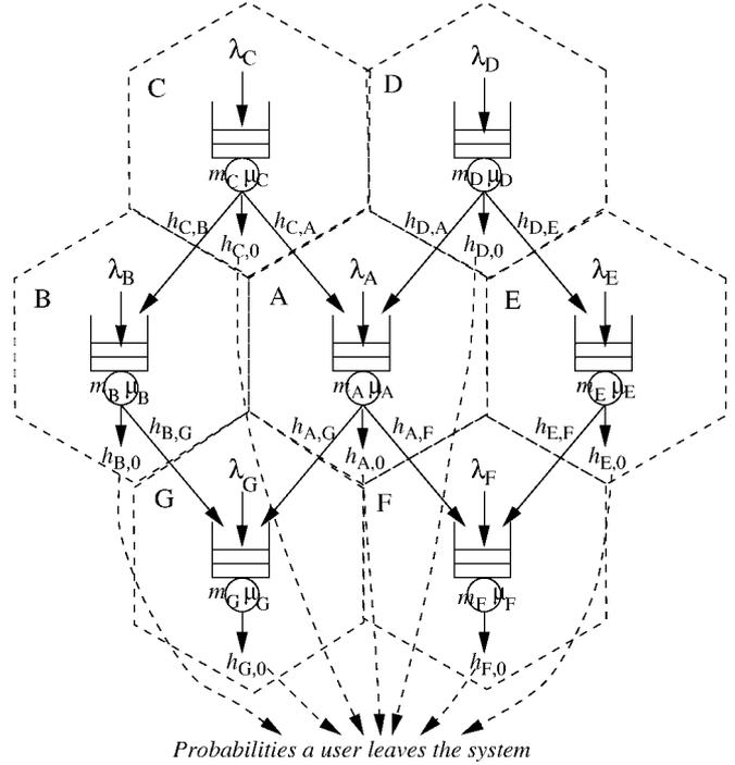
Figure 8. Queueing network model for spotbeams.
