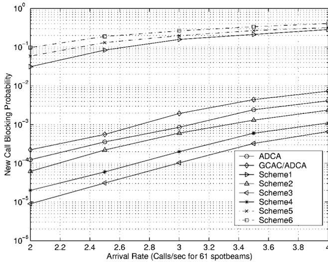
Figure 11. New call blocking probabilities ( $C = 190$ ).
