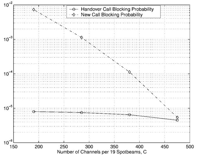
Figure 13. The effect of the number channels on the new call and handover blocking probabilities in GCAC/ADCA scheme (4 calls/s for 61 spotbeams).
