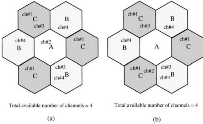
Figure 7. Example of dynamic channel allocation in spotbeams: (a) channel # 2 can be assigned in spotbeam A; (b) no channel can be assigned in spotbeam A ( $C = 4$ ).
