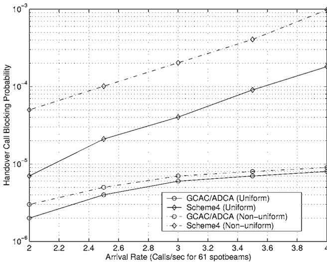
Figure 15. The handover call blocking probabilities (traffic pattern comparison).
