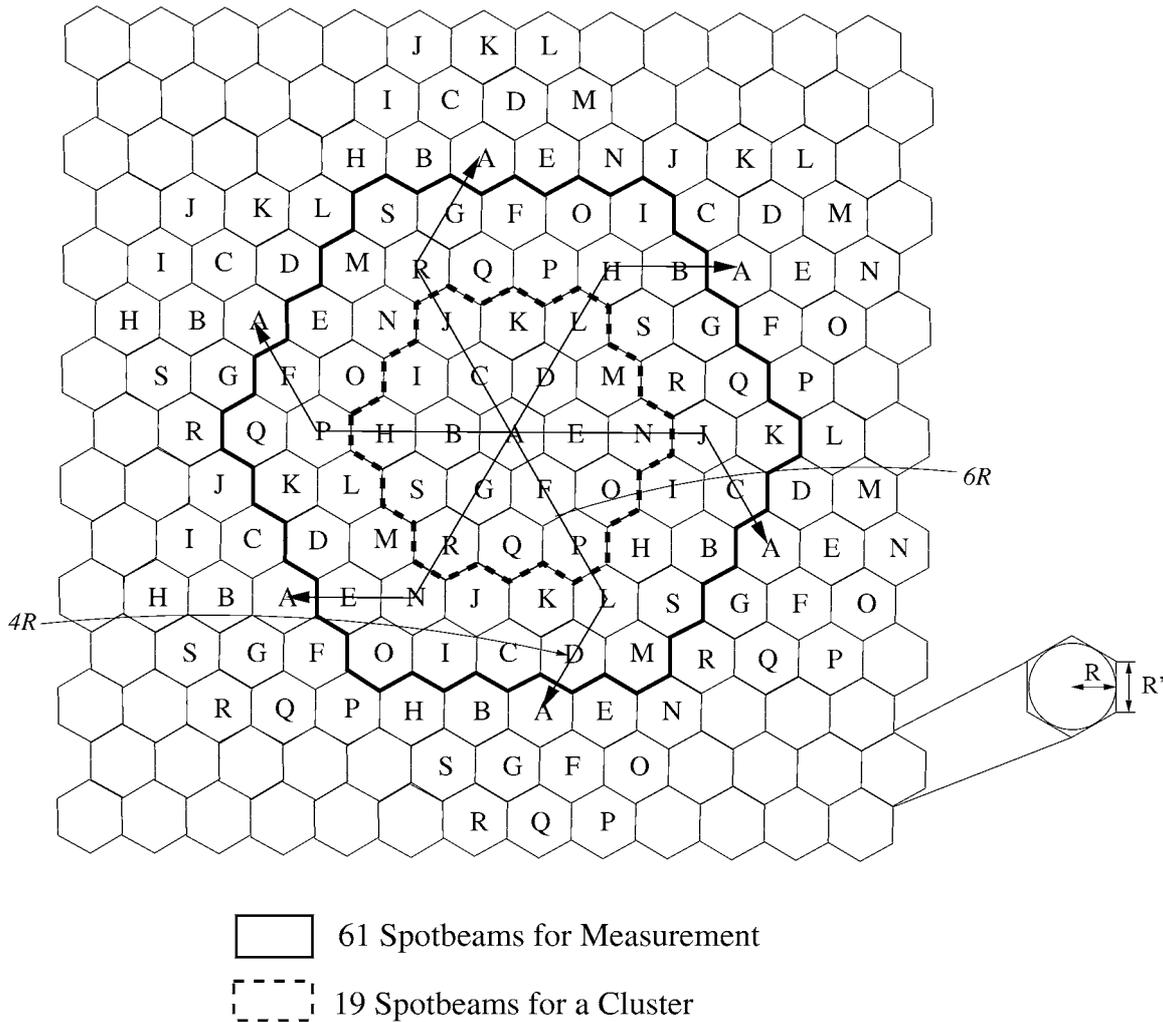
Figure 10. Cellular architecture in simulation.
