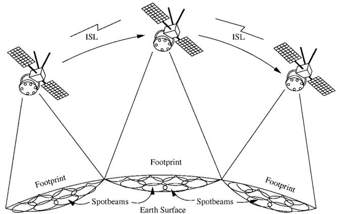
Figure 1. Spotbeams of LEO satellites.
