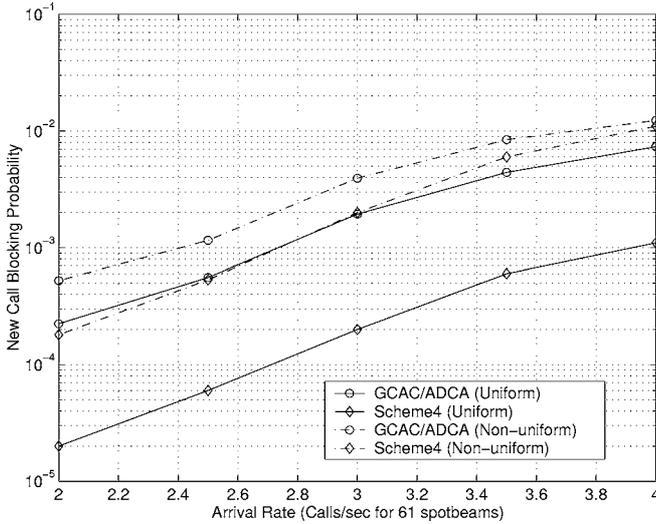
Figure 14. New call blocking probabilities (traffic pattern comparison).
