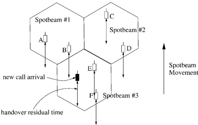
Figure 3. Illustration of ADCA scheme.
